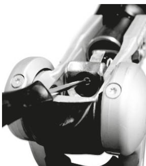
Fig 4. Remove head cap screw
